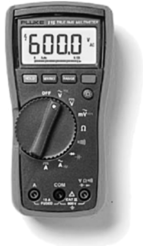
Figure 16.9 Handheld digital multimeter. Reproduced with permission of Fluke Corporation.
