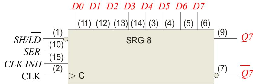
The clock ( $CLK$ ) and clock inhibit ( $CLK\ INH$ ) lines are connected to a common OR gate, so either of these inputs can be used as an active-LOW clock enable with the other as the clock input. Data is loaded *asynchronously* when  $SH/\overline{LD}$  is LOW and moved through the register *synchronously* when  $SH/\overline{LD}$  is HIGH and a rising clock pulse occurs.
