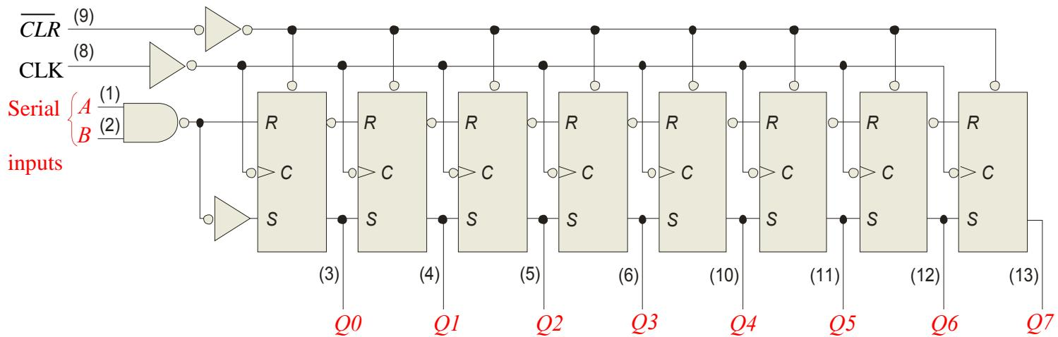
One of the two serial data inputs may be used as an active HIGH enable to gate the other input. If no enable is needed, the other serial input can be connected to  $V_{CC}$ . The 74HC164A has an active LOW asynchronous clear. Data is entered on the leading-edge of the clock.
