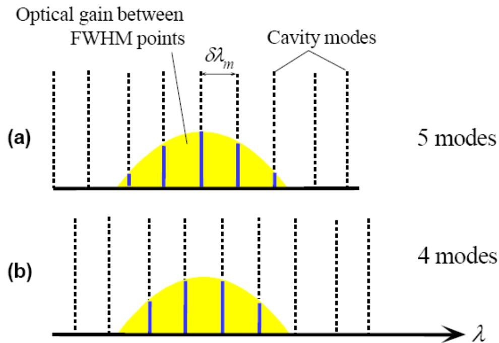
Number of laser modes depends on how the cavity modes intersect the optical gain curve. In this case we are looking at modes within the linewidth  $\Delta\lambda_{1/2}$ .
