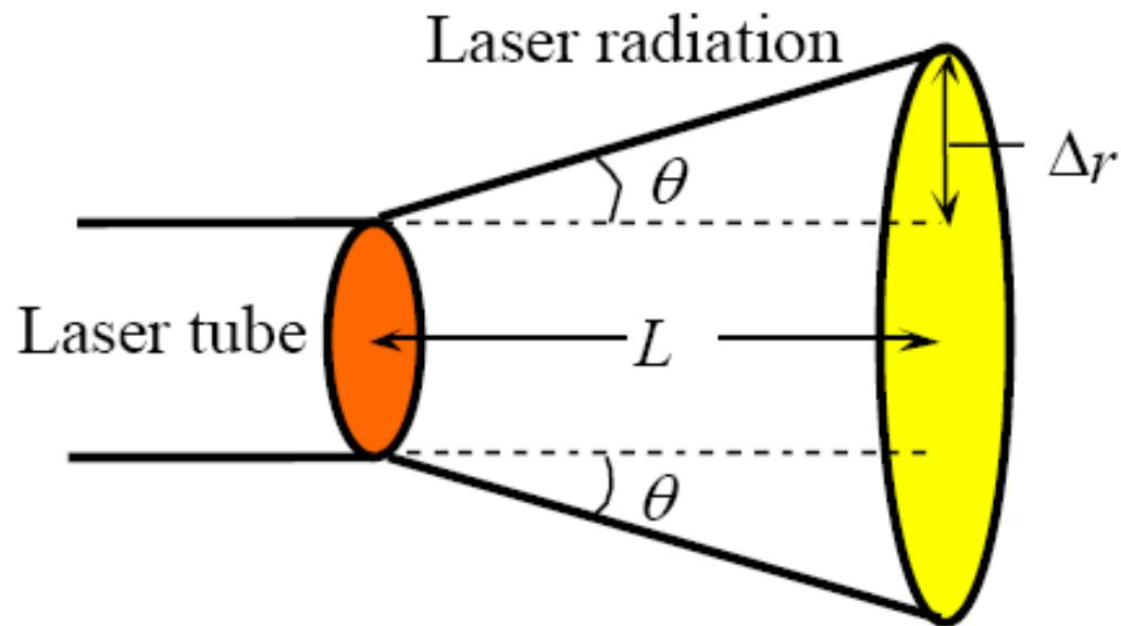
The output laser beam has a divergence characterized by the angle  $2\theta$  (highly exaggerated in the figure)
