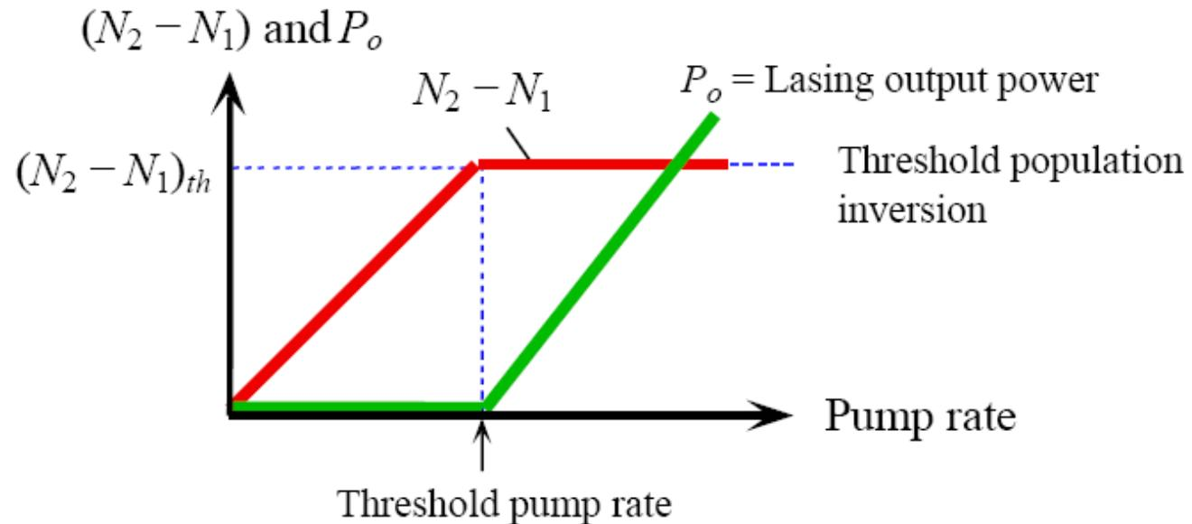
Simplified description of a laser oscillator.  $(N_2 - N_1)$  and coherent output power ( $P_o$ ) vs. pump rate under continuous wave steady state operation.
