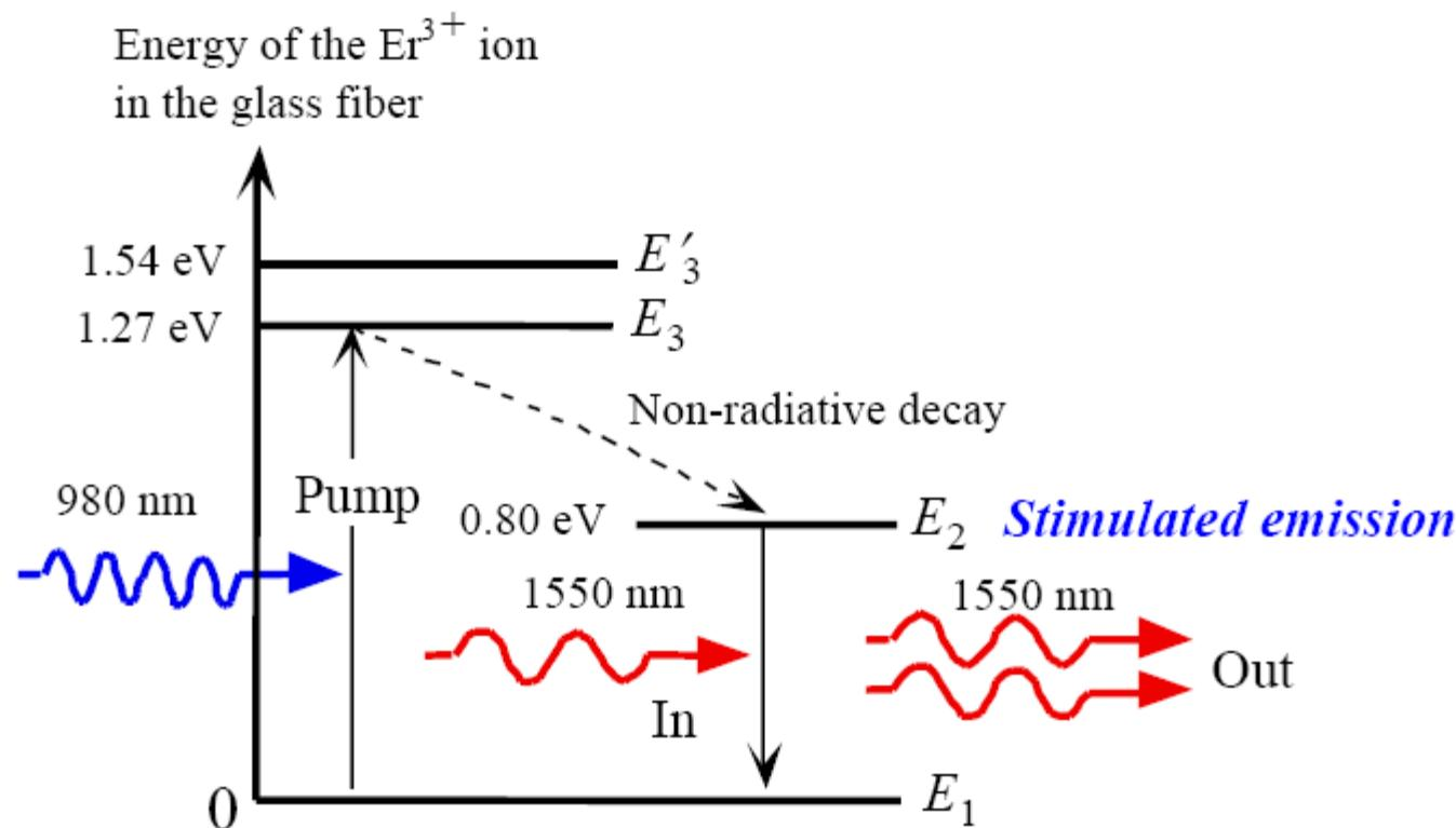
Energy diagram for the  $\text{Er}^{3+}$  ion in the glass fiber medium and light amplification by stimulated emission from  $E_2$  to  $E_1$ . Dashed arrows indicate radiationless transitions (energy emission by lattice vibrations)
