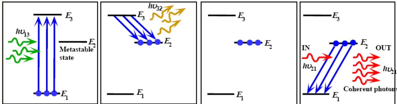
Atoms in the ground state are pumped up to the energy level  $E_3$  by incoming photons of energy  $h\nu_{13} = E_3 - E_1$ .
