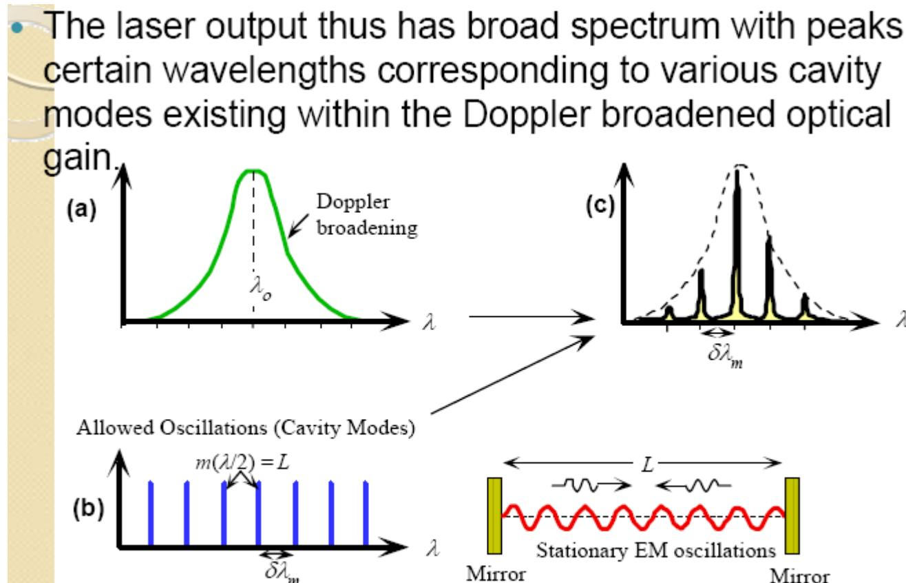
The output spectrum is determined by satisfying (a) and (b) simultaneously.
