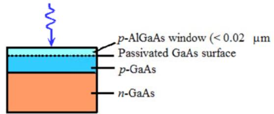
AlGaAs window layer on GaAs passivates the surface states and thereby increases the low wavelength photogeneration efficiency
