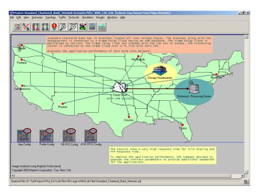
The PVCs connecting all the branches to the frame cloud are configured with a CIR of 64 kbps. Even though the contract parameters agreed between the bank and Verizon can be accomplished by a 128 kbps access link, Verizon has a 256 kbps access link running from the regional routers to the frame cloud to anticipate future upgrade or additional bank branches. The PVC from
